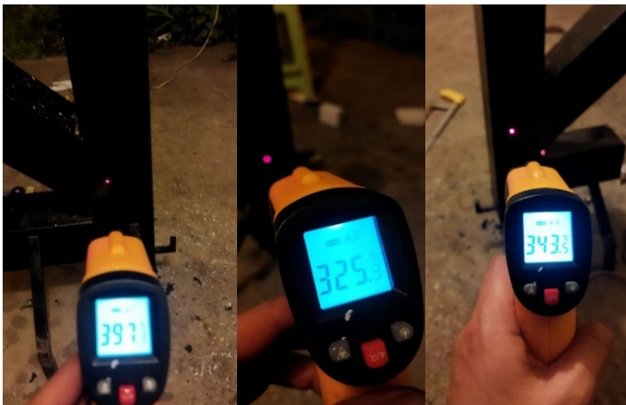
Figure 9. Measurement of temperatures in the three walls of the combustion chamber
