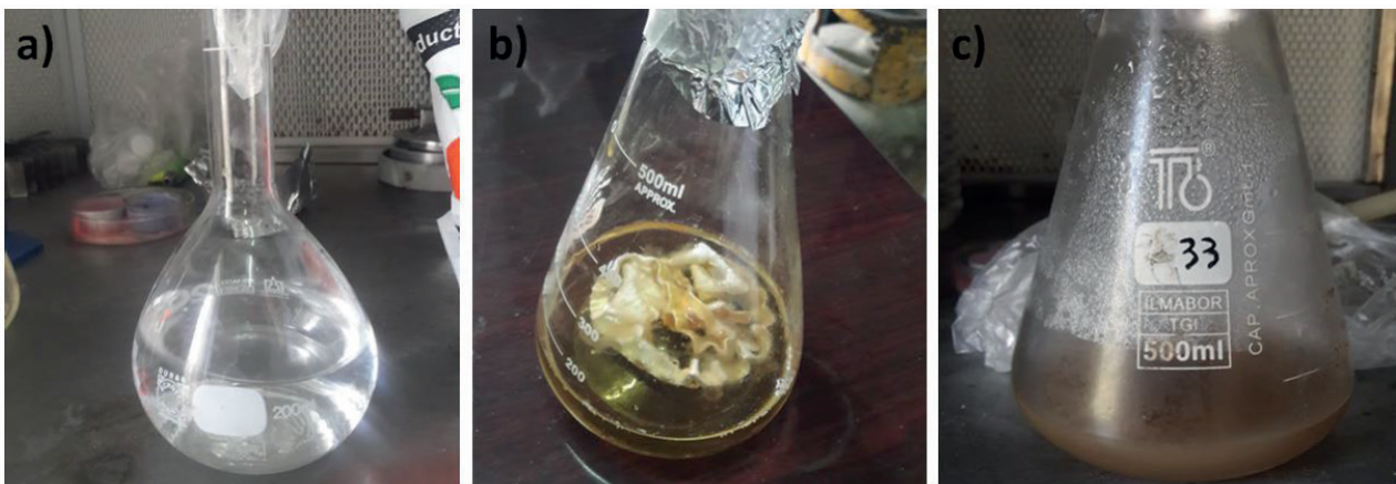
Figure 2. Synthesis of AgNPs: a) AgNO 3 (1 mM) solution; b) A. terreus biomass (50 mL); c) Color alteration of filtrate after incubation in the dark.
