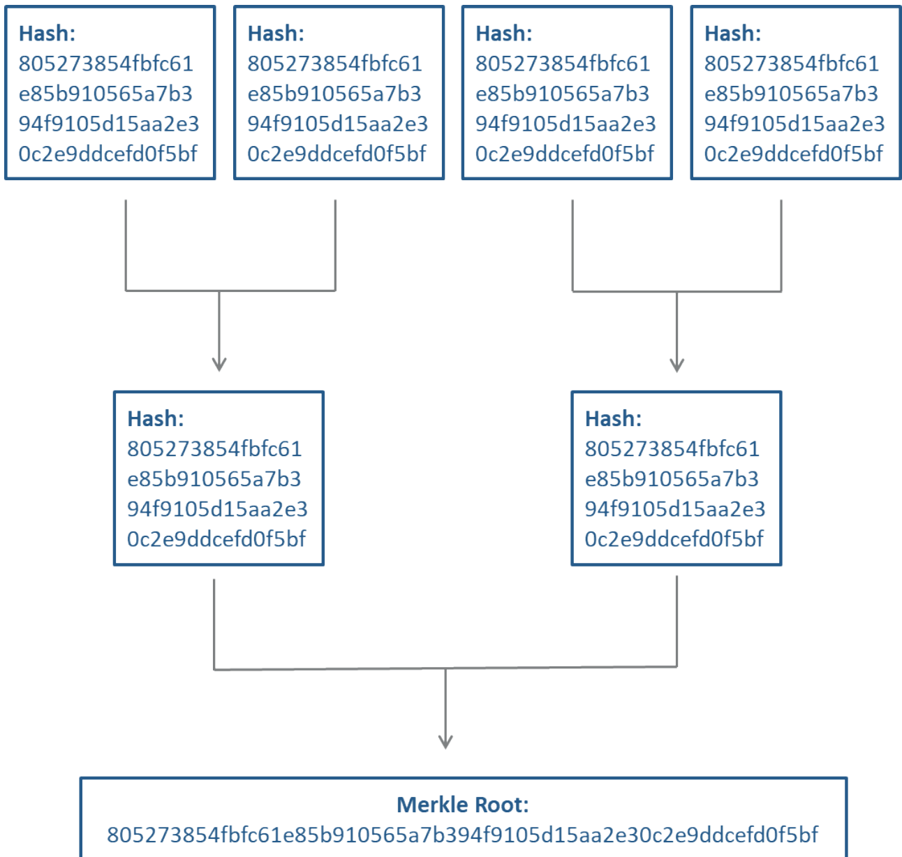
Figure 7. Merkle tree structure formed by hashes of different transactions.
