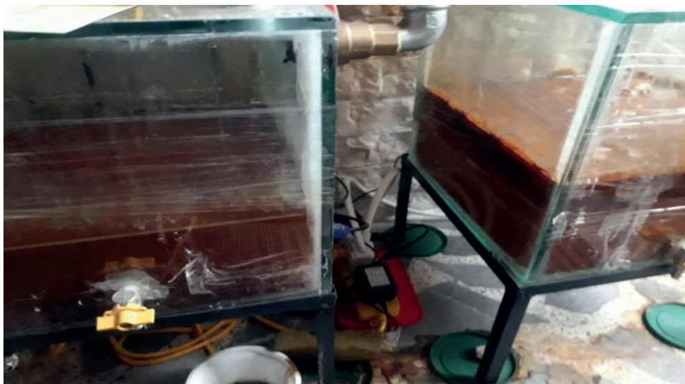
Figure 2. Anaerobic reactors and the fermentation process.
