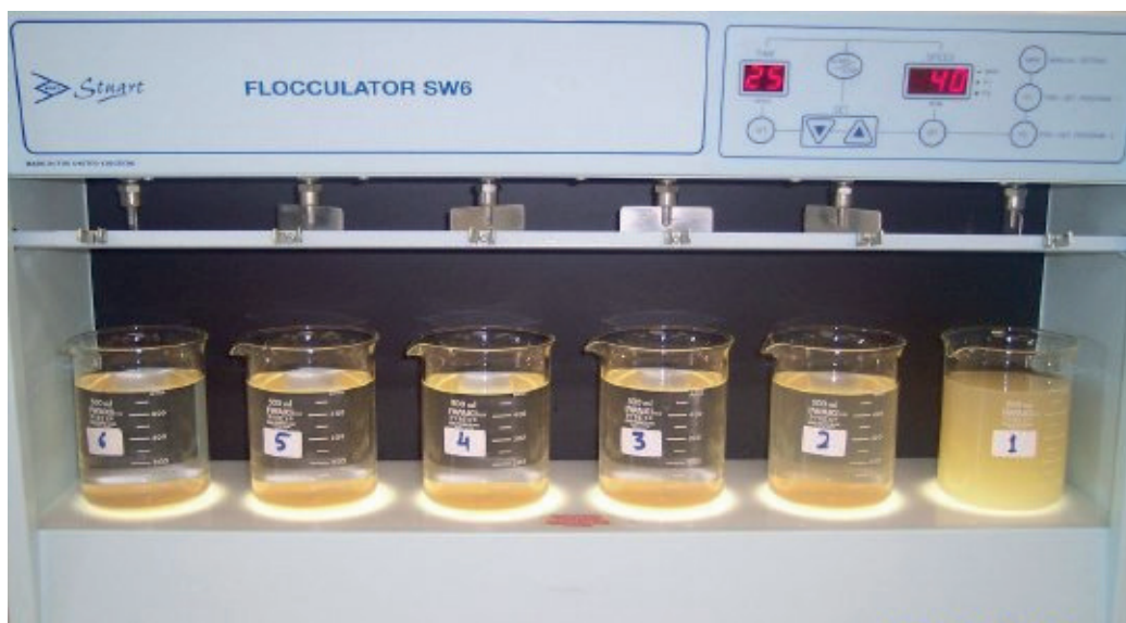
Figure 2. A traditional jar test device was owing for the treatment of turbid water.
